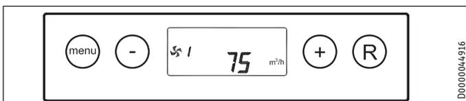
The appliance then runs according to the stage switch setting. If no stage switch is connected, the appliance always runs in fan stage 1.
