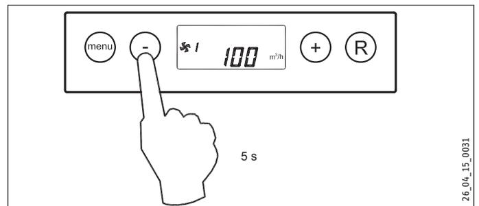
► Switch on the appliance by pressing the minus button for 5 seconds.
