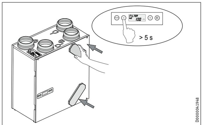
► Assemble the two filter flaps.
