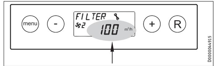
The selected air flow rate of the supply air and extract air fans is displayed.
