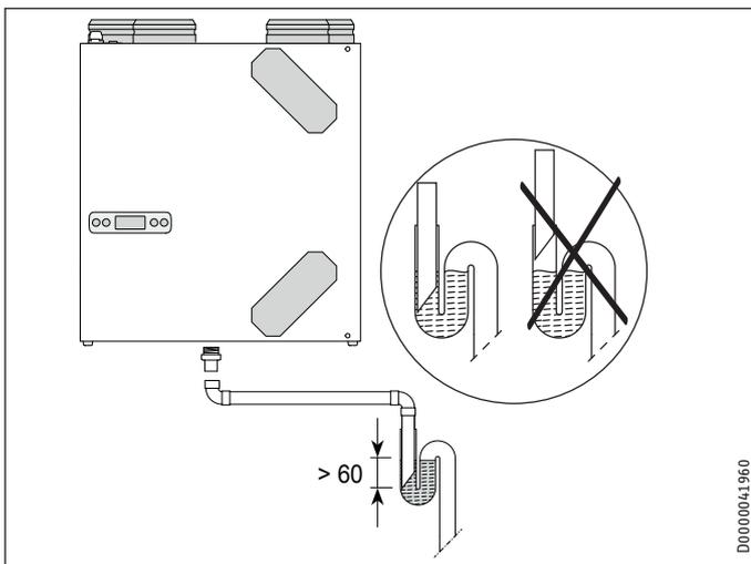
The condensate drain is routed through the floor plate. The condensate must drain away via the domestic sewer system.
