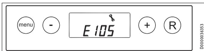
If the appliance detects a blocking fault code, it stops. The permanently illuminated display shows the fault symbol (spanner) together with a fault code.
