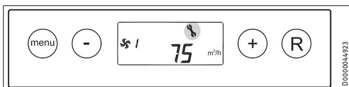
If the appliance detects a non-blocking fault code, it continues to operate with limited functionality. Non-blocking faults are displayed with the fault symbol (spanner).
