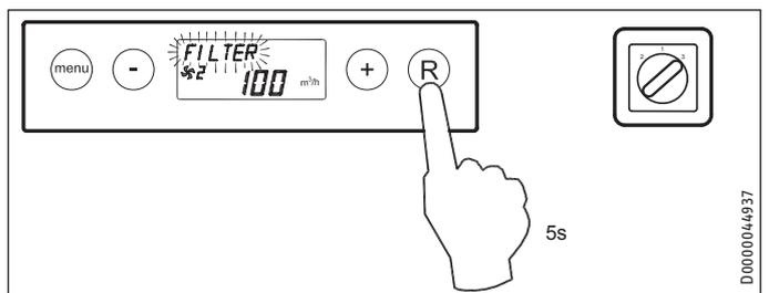
► After cleaning or replacing the filters, hold down the R key for 5 seconds to reset the filter display.
