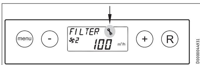
If the appliance detects a fault, a flashing fault symbol (spanner) is displayed, possibly together with a fault code. The appliance differentiates between a fault, where the appliance continues to operate with limited functionality, and a blocking fault, where both fans are stopped. In the event of a blocking fault, the settings and read-out menus are also switched off and access is restricted to the service menu.
