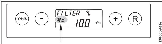
A fan symbol is displayed when the supply air fan and the extract air fan rotate. The fan symbol is not visible when the fans are at a standstill.
