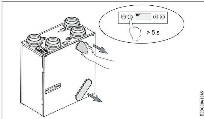
► Press and hold down the minus button for 5 seconds to switch off the appliance.
