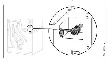
▶ Drain the DHW cylinder via the drain valve.
