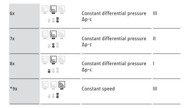
(\*) Pressing the button for the 9th time returns to the basic setting (constant speed / characteristic curve III).
