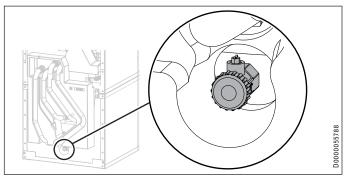
▶ Drain the buffer cylinder via the drain valve.
