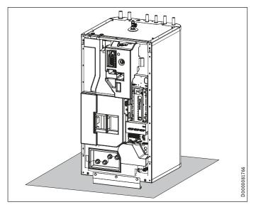
► Place the upper section of the appliance on a base to prevent damage.
