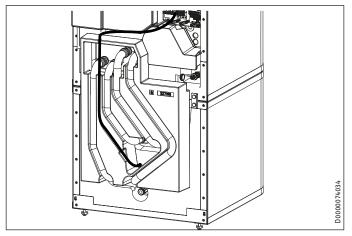
► Release the sensor lead from the guide groove in the insulation segment.
