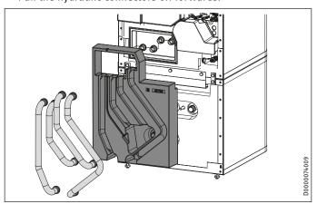
► Remove the 4 hydraulic hoses and the insulation segment.
