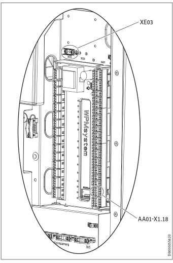
► Detach the plug of the electronic assembly for operation (AA01-X1.18) and the earth connection (XE03) on the heat pump manager.
