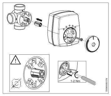
► When installing the servomotor, ensure the drive cam is positioned correctly.
