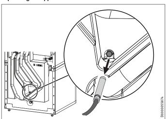
▶ Pull the "heating sensor" out of the buffer cylinder.
