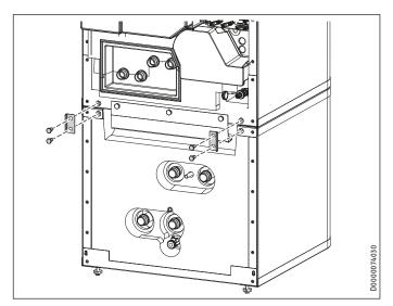
▶ Release the 4 screws on the tabs at the front of the appliance.
