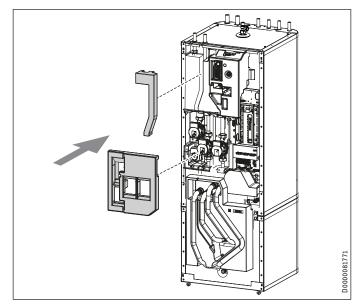
► Insert the EPS profiles on the HSBC side.
